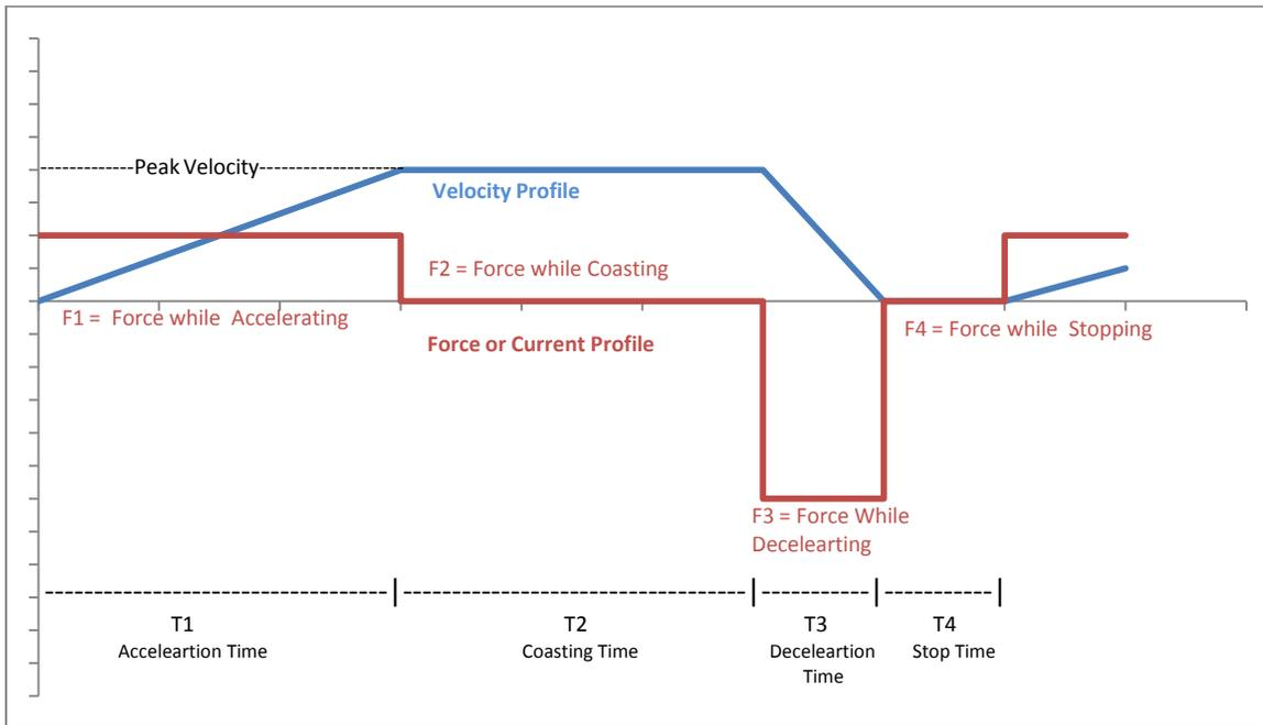
$$X = 0.5 V_{peak} (T_1 + 2T_2 + T_3)$$
